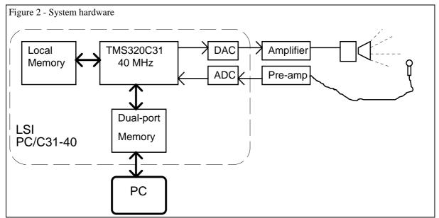
The software was written on a PC, in a couple of days, using the SigLib library. The DSP code was compiled for the TMS320C31, while a host program was also written for the PC, to allow it to control the DSP functionality.
